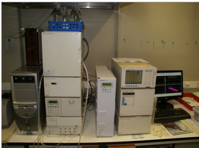
Fig. 13 – Shimadzu HPLC system with diode array detector (DAD).
