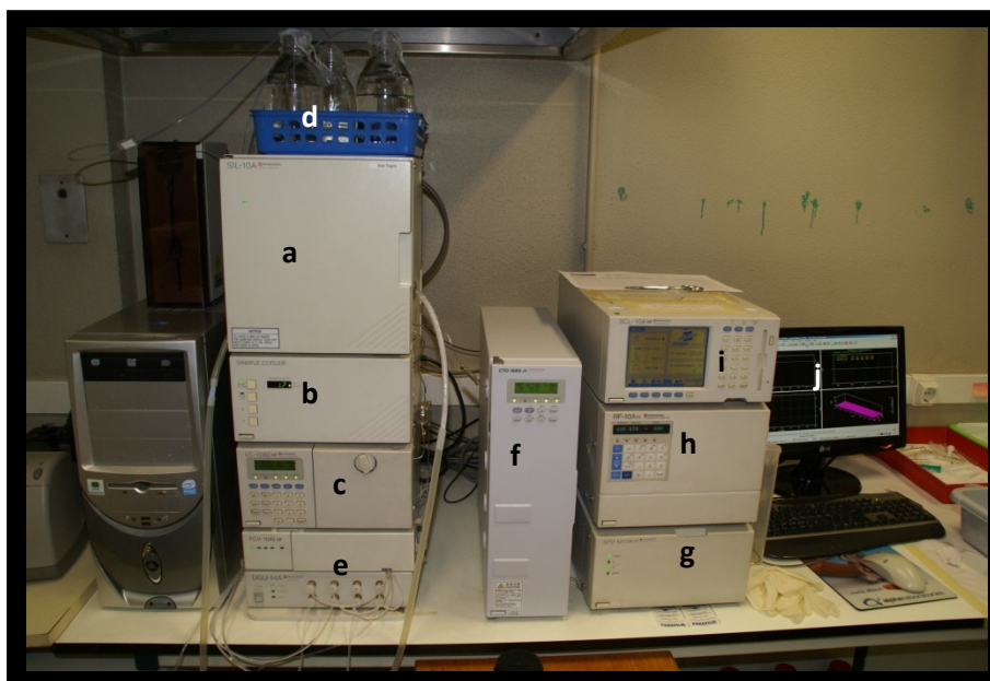
Figure 7 – Extracts are put into the auto-sampler (a), which injects automatically the samples into the HPLC system, maintained at 1°C by a cooler (b) which are sent into the chromatographer (c). Solvents (d) are sent through the degasser (e) to the chromatographer (c). From here samples diluted in solvents go through the separation C18 column (f) where they bind and come out at different times. As the different pigments leave the column absorbance is read by the photodiode array detector (g) and chlorophyll fluorescence is
